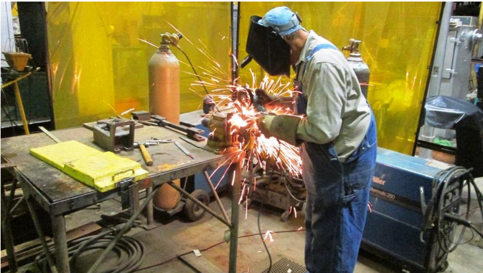
Cliff uses a grinder to finish work on the man-lift's battery box modifications
